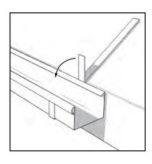
Fix the pipe brackets at a maximum of 2 meters.
