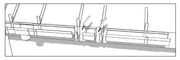
If you use glue-fittings, the gutter can be glued into the fittings. Make sure the surface is clean before applying the glue. The seam in which the gutter is stuck, must be filled with glue. Afterwards, apply some additional glue along the inside seam.
