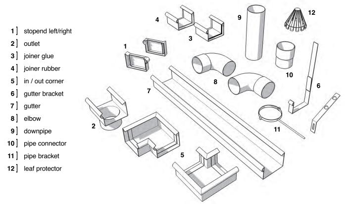
Determine the position of the outlet. That is automatically the lowest point. After that, you can also determine the highest point. Install a bracket at the lowest and one at the highest point. A string secured between both brackets will assist in installing the remaining hangers.
